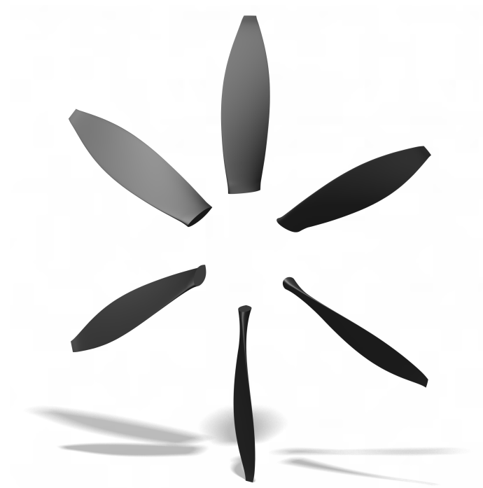
Figure 2.11: 3D model of baseline propeller created in CATIA V5.
